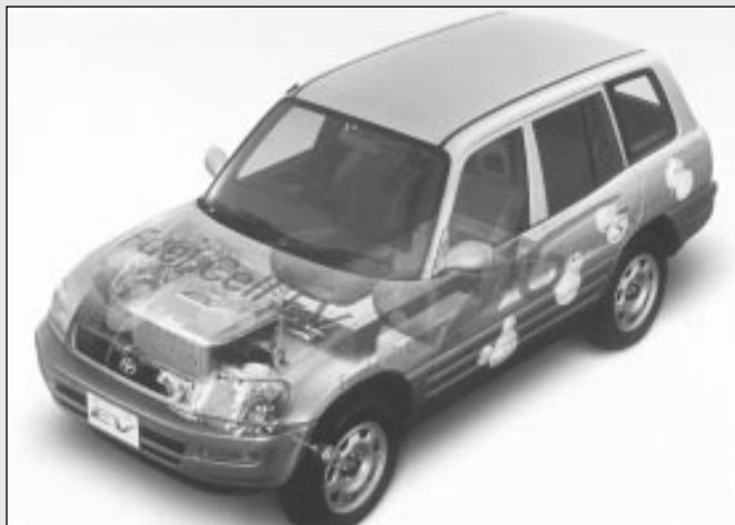
Toyota says its new non-polluting car runs on electricity generated by a reaction between hydrogen and oxygen.
